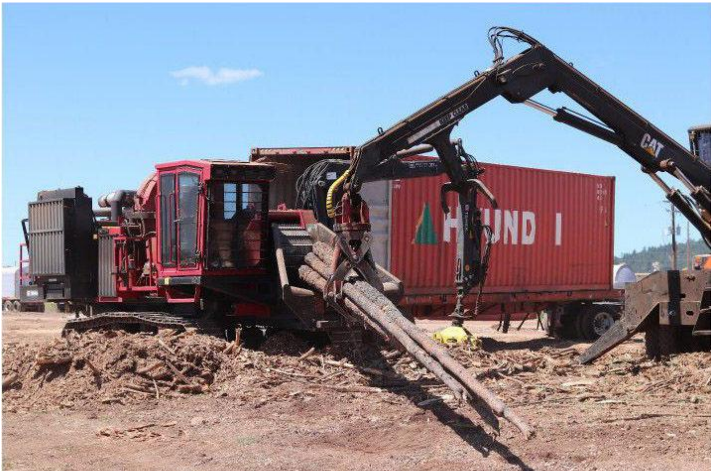
Log loader feeding logs into the tracked chipper.
