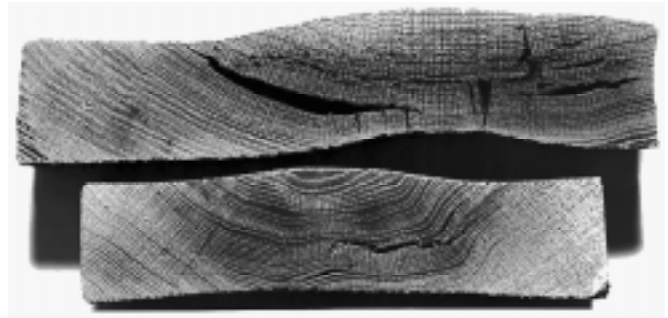
Figure 51—Shake is failure that follows the growth rings.
