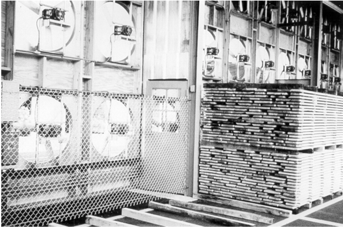
Figure 3—Fan shed air dryer draws air through the stickered packages of lumber.
