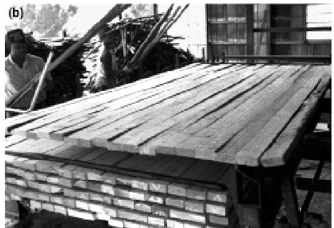
Figure 37—Semiautomatic stacker; (a) crews lay the stickers in place (b) at which time the stacker places a layer of lumber on the stickers.
