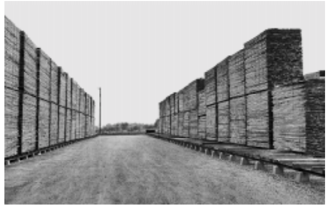
Figure 27—The main features of well-constructed pile foundations and lumber piles in an air-drying yard.
