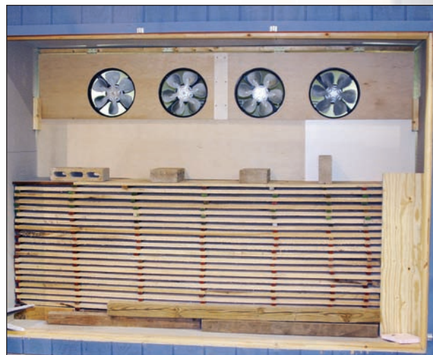
Figure 4: The hinged baffle houses the four fans and controls the airflow.
