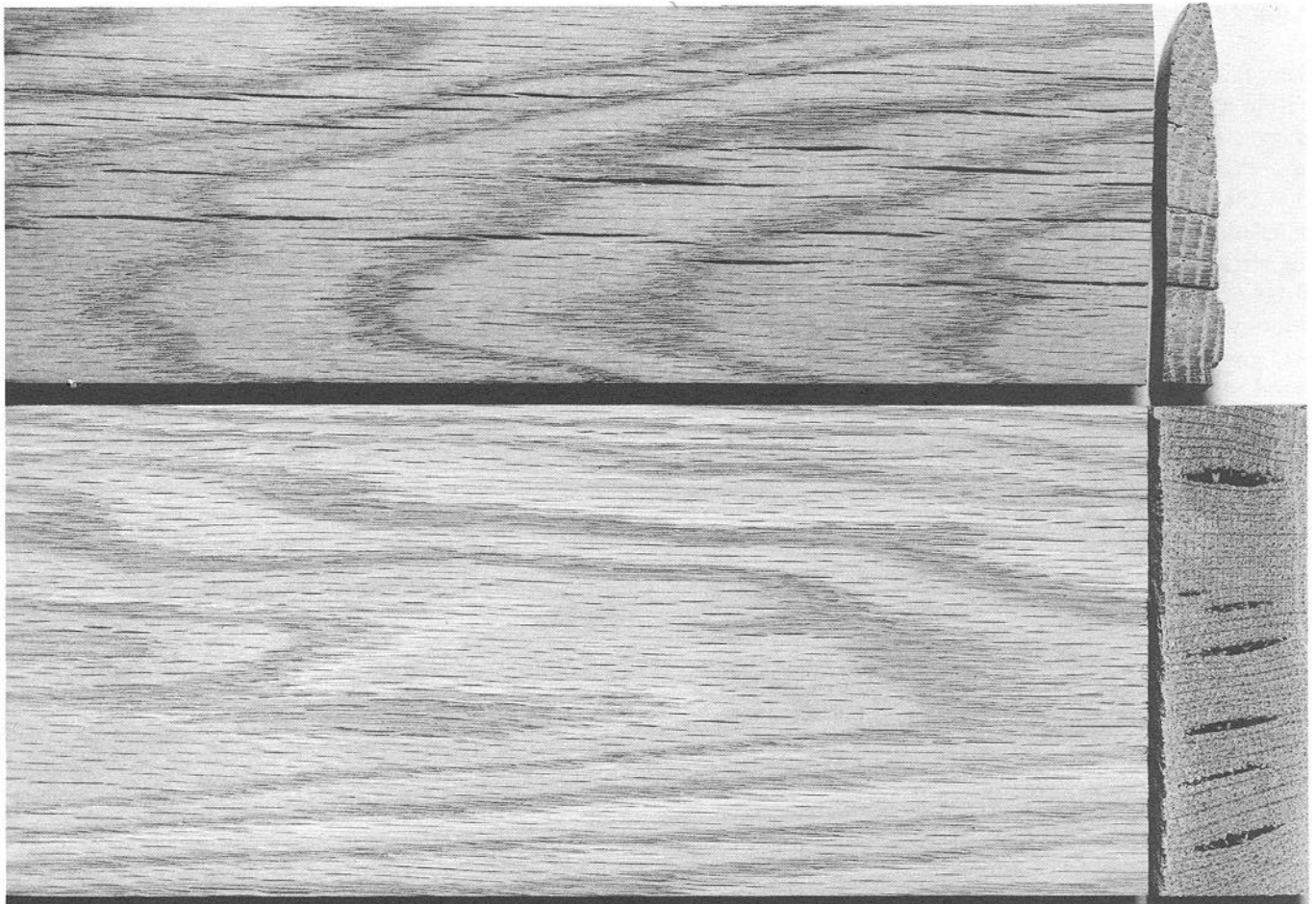
Figure 8-7—Honeycomb that does not appear on the surface of a planed red oak board (lower) does appear
