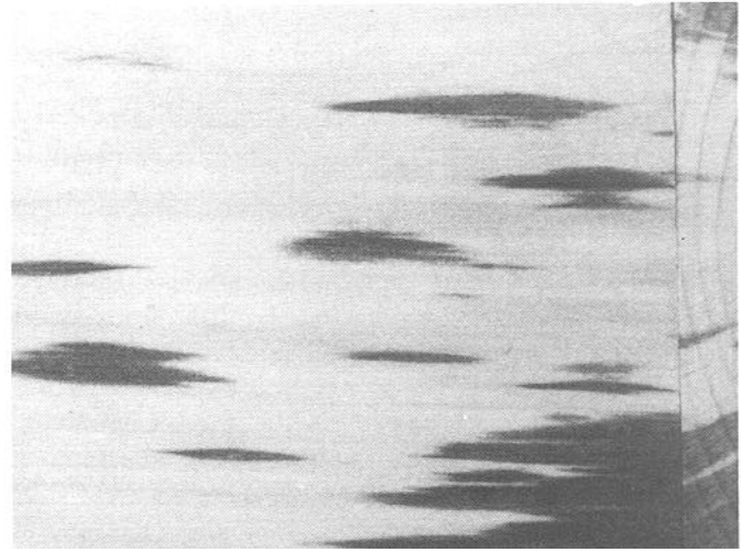
Figure 8-18—Surfaced board of eastern white pine revealing blue stain that developed during the early stage of dehumidification drying. The lumber was from winter-cut Jogs and was not chemically treated. (M88 0160)
