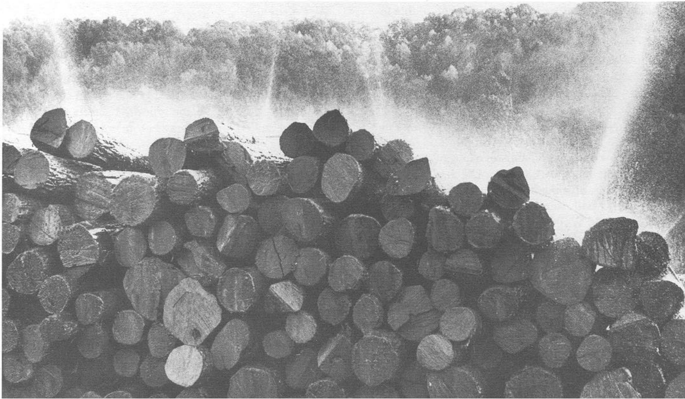
Figure 10-7—Water sprinkling of decked hardwood logs. A fine mist effectively covers log surfaces and ends. (M 144876).
