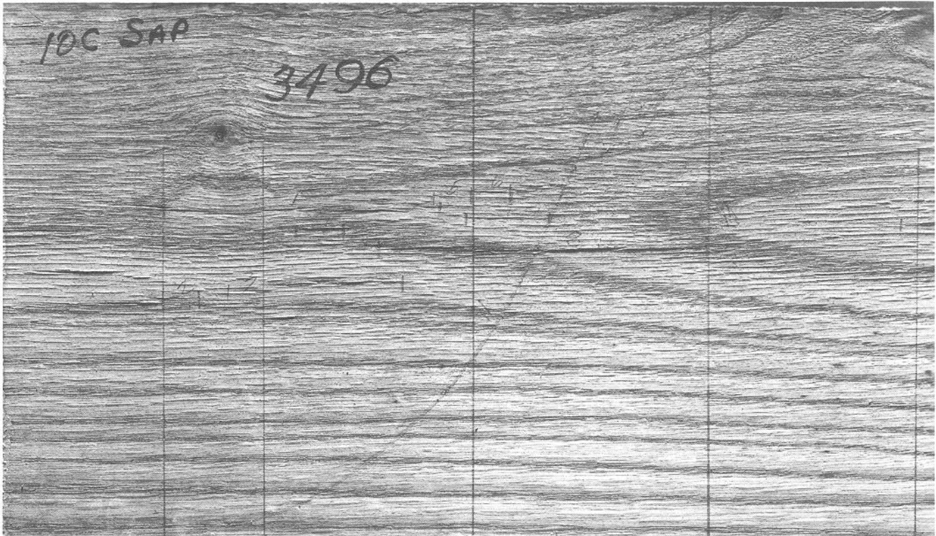
Figure 8-1—Surface checks in cherrybark oak. (M 137194)
