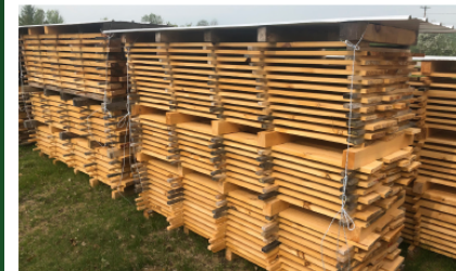
Figure 1. Pile covers in an air-dry yard help preserve the quality and value of the lumber by protecting the lumber from the elements. Photo source: Coos Forest Products.
