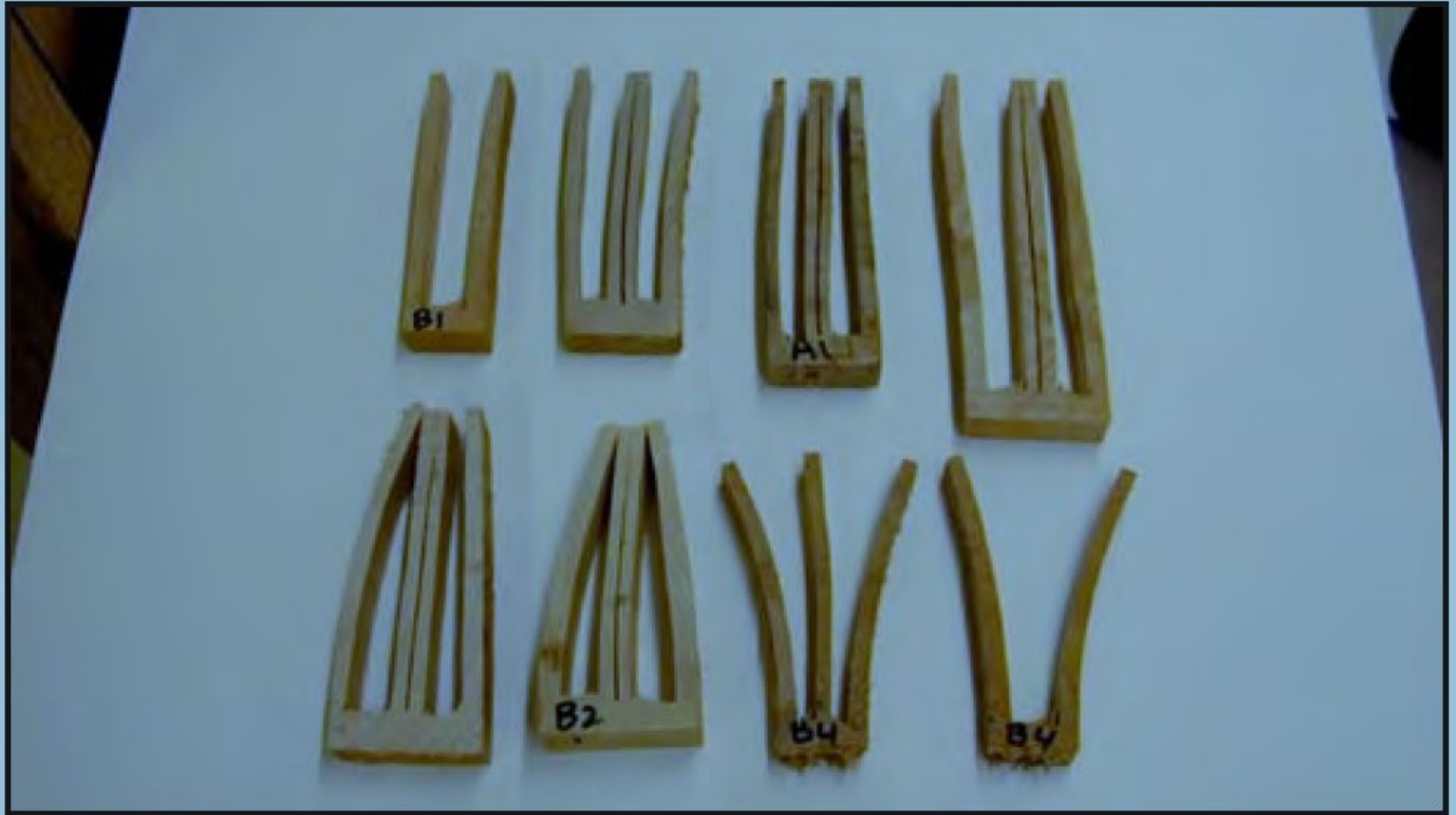
Figure 11-22. Stress or casehardening test in kiln-dried lumber. Prong tests in the top row show no stress. The two samples on the bottom left show casehardened lumber, while the two on the right show reverse casehardening.
